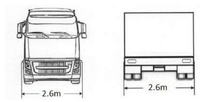
**Note:** Side cargo overhangs from the two sides of the vehicle cannot exceed 30cm.
